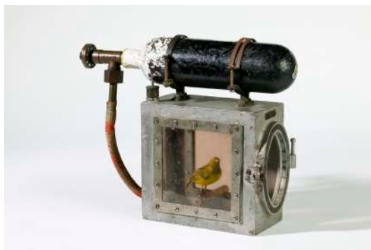
Figure 3: Cage for reviving canary, with oxygen cylinder, made by Siebe Gorman & Co. Ltd, London.
